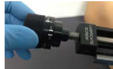
I. Confirm zero alignment of knob and turn knob clockwise to apply tension.
